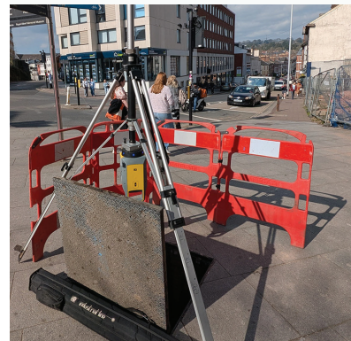
At the manhole site, the Trimble X7 was used on an inverted tripod to link the above and below ground surveys
